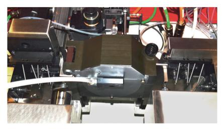
The two back machining units are identical. The units consist of a counter collet which is mounted on a table with cross slides. The work piece in the counter collet can be machined with two axial spindles (18'000 min<sup>-1</sup>) and one cross spindle (18'000 min<sup>-1</sup>). To increase the drilling speed or to index the part the machine can be equipped with two C-axis (10'000 min<sup>-1</sup>)
